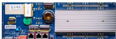
RS485 * Communication between battery and server Band rate:9600bps RS485 Interface Communication between parallel packs or BMS and PC Band rate:9600bps
