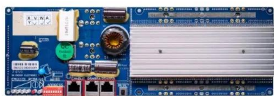
RS485 Communication between battery and inverter Baud rate: 9600bps RS485 Interface Communication between parallel packs or EMS and PC Baud rate: 9600bps
