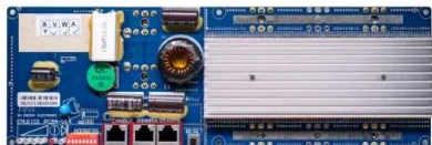
ES485 * Communication between battery and inverter Band rate: 9600bps ES481 Inverter Communication between parallel packs or EMS and PC Band rate: 9600bps
