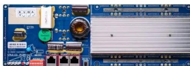
RS485 Communication between battery and server Band rate:9600bps RS485 Interface Communication between parallel packs or EMS and PC Band rate:9600bps
