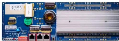
ES485 Communication between battery and inverter Baud rate:9600bps ES483 Interface Communication between parallel packs or BESS and PC Baud rate:9600bps
